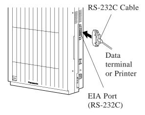
Insert the RS-232C cable into the VPS with the connector indicating the same direction.
