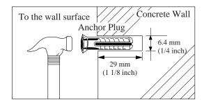
3 Install the 3 screws into the anchor plug.
