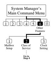
Each Class of Service defines a set of services available for Subscribers. A maximum of 64 Class of Service can be established. You can set each Class of Service from a telephone. For the details of individual description, see **Setting Class of Service Parameters** in Chapter 4. COS No. 63 and No. 64 have been assigned to the Message Manager and the System Manager respectively.
