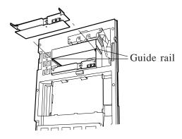
5. Press the left and right card latches firmly, then fix the grounding strap to the unit with a screwdriver.
