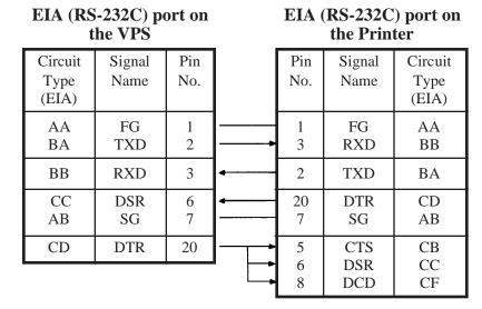
The pin configuration of the EIA (RS-232C) connector is as follows.
