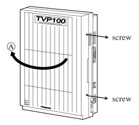
**Note:** The screws are attached to the front cover with springs so that they will not be lost.
