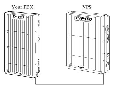
3 Connect the telephone cord to the extension port of the PBX.
