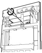
**4.** Insert the optional Port card into the SLOT 2 along with the guide rails.
